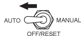
Figure 52. MPEC Control Switch (AUTO)
